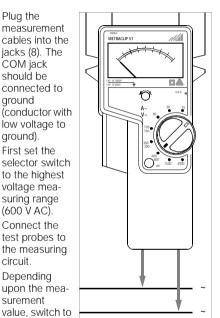
suring range with higher resolution. If possible, pointer deflection should be greater than one third of the overall scale.
